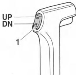
1. Power trim and tilt switch
